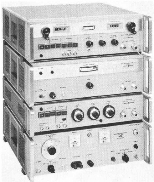
Fig. 3. Combinations of recent -hp- instruments showing flexibility of modular enclosure system designed and now used by -hp- . Enclosures are \frac{1}{3} , \frac{1}{2} and full EIA rack width, are suited to bench, rack or, with special carrying covers, to field use.
